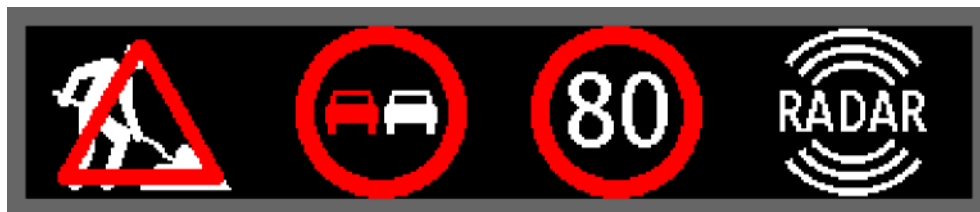
Figure 19: Maximum number of elements on VMS, 4 x class 1 (Example)
