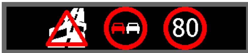
Figure 20: Maximum number of elements on VMS, 2 x class 1 and 1x class 2 (Example)
